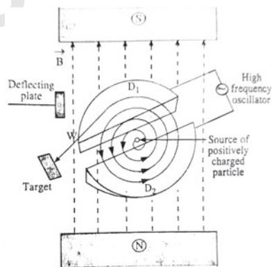
**Construction :** It consists of two hollow D-shaped metallic chambers  $D_1$  and  $D_2$  called dees. These dees are separated by a small gap where a source
