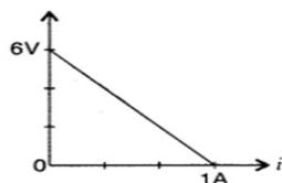
Ans: Total emf of three cells in series = P.D corresponding to zero current = 6V
