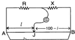
Hence, the galvanometer and cell are interchanged, the condition for a balance bridge is still satisfied. Therefore, the galvanometer will not show any deflection.
