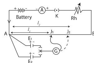
When the key K is closed, a constant current flows through the potentiometer wire. By closing
