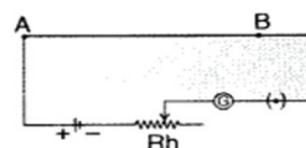
Principle : The basic principle of a potentiometer is that when a constant current flows through a wire of uniform cross-sectional area and composition, the potential drop across any length of the wire is directly proportional to that length.
