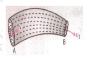
Let  $a_1$ ,  $v_1$  and  $\rho_1$  be area of cross section, velocity of the flow of liquid and density of the liquid at point A' of tube and  $a_2$ ,  $v_2$  and  $\rho_2$  be area, velocity and density of the liquid at point B' of the tube. Volume of liquid entering per second at  $A = a_1.v_1$  and at  $B = a_2.v_2$
