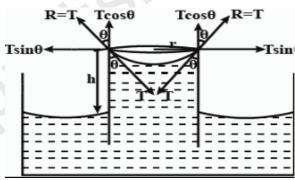
Consider a capillary tube of radius r partially immersed into a wetting liquid of density  $\rho$ . Let the capillary rise be h and  $\theta$  be the angle of contact at the edge of contact of the concave meniscus and glass figure. If R is the radius of curvature of the meniscus then from the figure,  $r = R \cos \theta$ .
